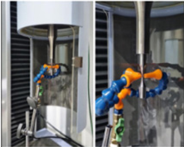
Figure 7: DIN34CrNiMo6 steel specimen under fully reversible loading.
