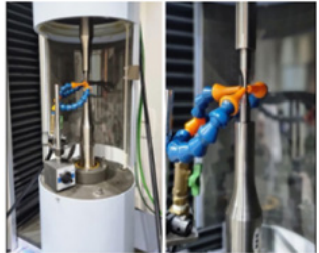
Figure 8: DIN 34CrNiMo6 steel specimen under partially reversible loading.
