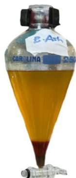
Figure 2: Biofuel using calcined banana ash as catalyst.
