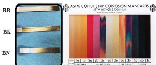
Figure 8: Copper strip test for the prepared biofuels.
